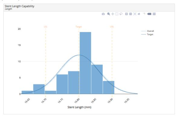
The Overall curve shows that the process is centered much better than it was in week 1. However, the distribution seems to be more spread out than it should be. The is especially true on the left side.
