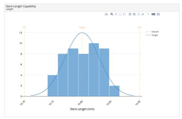
The capability graph shows that the data are much more tightly grouped around the mean then they were in week 2. All the bars on the histogram are well within the spec limits.
