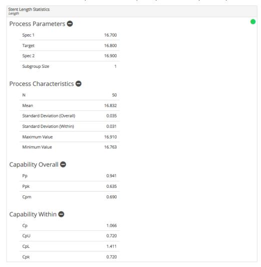
The Ppk and Cpk values indicate that the process is not very capable. In other words, based on the mean and variability of our sample, a high number of the parts produced by the process are not within the specification limits.
