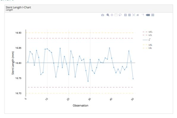
The I-chart looks good. The mean appears to be right on target. All the points are within the control limits and none of them failed any of the tests for special causes.
