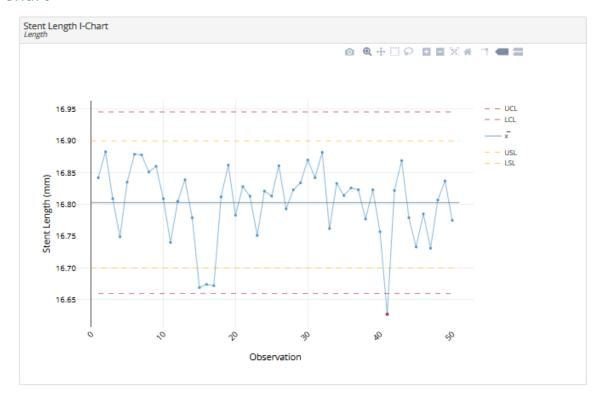
The good news is that the mean of the parts, indicated by the center line, is very close to the desired target of 16.80.
