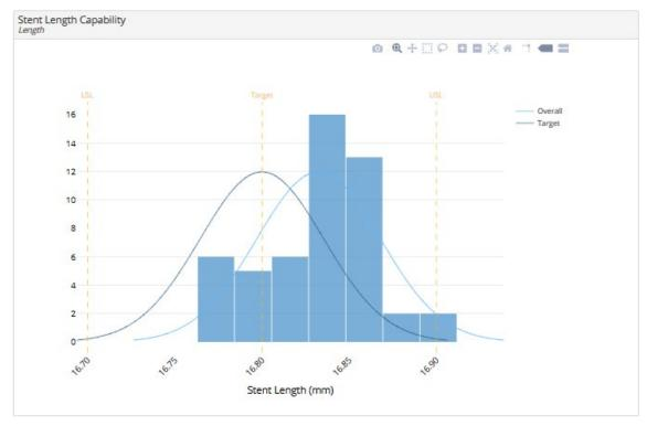
Each bar on the histogram indicates the number of sample values (y-axis) that fall within the indicated range of measurement values (x-axis). For example, the first bar on the left indicates there are 6 measurements in the sample that fall between 16.76 mm and 16.78 mm.
