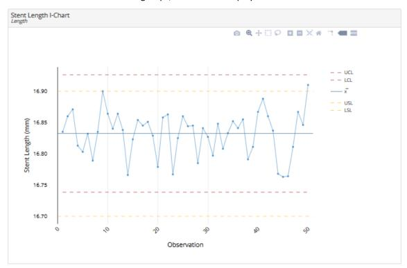
If your process is running smoothly, the points should vary randomly about the center line. All points should be between the upper control limit (UCL) and the lower control limit (LCL). In addition, TRENDABLE performs several tests on your data to help identify potential problems. Points that fail any of these "tests for special causes" are indicated with a red square instead of a blue circle.
