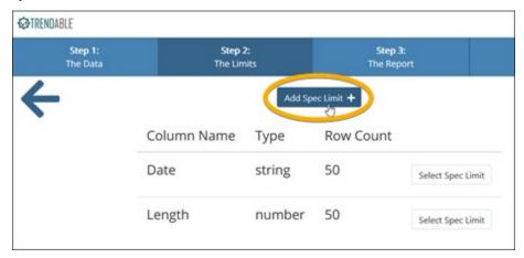
2. Enter a name for the spec limit, such as "Stent Length", then enter the units, the target, and the upper and lower limits as shown below.
